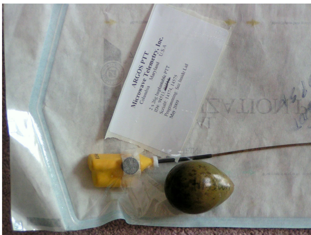
Fig. 1 Size and shape of an implantable satellite transmitter (in sterilized package) compared to a Black-tailed Godwit Limosa limosa egg. The dark object on the yellow transmitter body is a magnet that activates a reed switch, preventing transmissions until it is removed. The white object at the base of the antenna is a collar made of polyester fabric that served as an anchor point for suturing to stabilize the transmitter within the bird’s body
