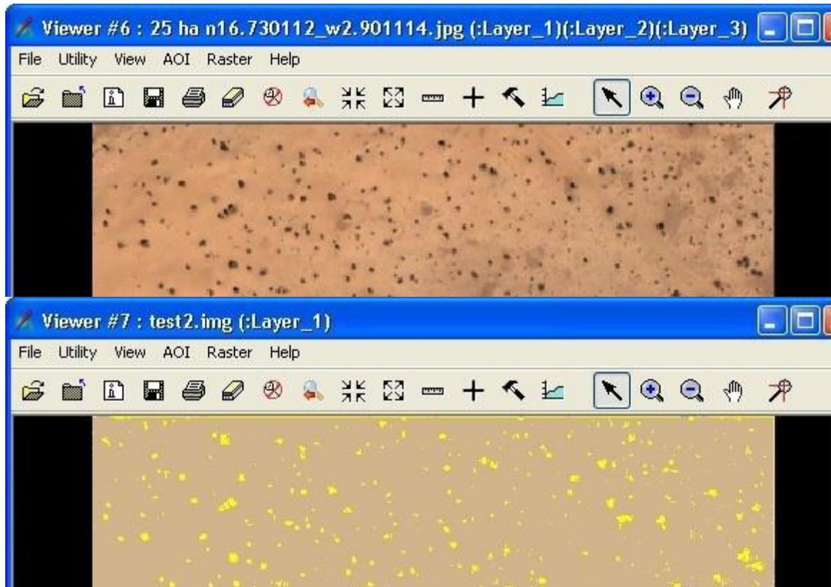
**Fig. 16.** Google image (width 500 m) of an Acacia forest in northern Mali, converted into an ArcGis- shapefile, allowing us to quantify semi-automatically tree density and canopy.
