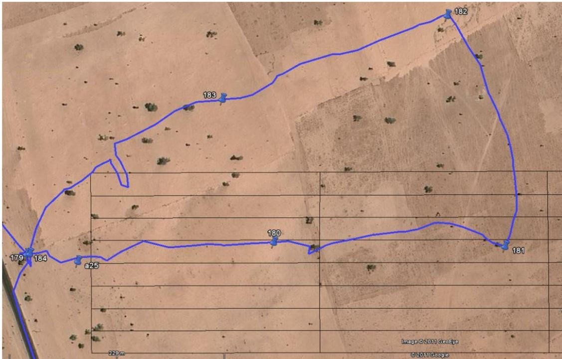
**Fig. 13.** The grid with the black lines gives the pre-selected plot(250 x 25 m each) for site “a25”. The blue line shows the actual GPS-track. The waypoints indicate where the data were split up into five different transects being each 250 m long and 50 m wide.
