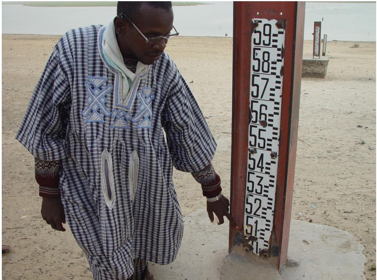
*Thanks to DNH the daily water level is known for several hydrological stations in the Inner Niger Delta. The picture shows Navon Cissé (DNH) and the scale of Akka.*
