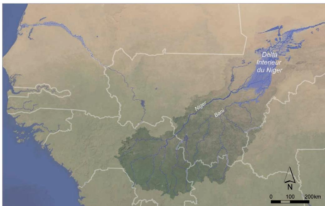
The catchment area of the Niger and Bani is given in bright colours. The flooding of the Inner Niger Delta is determined by the inflow from both rivers, which in turn relates to the rainfall experienced 600-1200 km away in the same year and the ground water table in the Upper Niger Basin such as determined by the rainfall during the preceding years.
