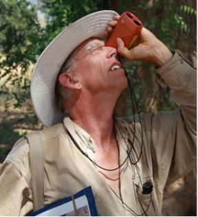
**Fig. 12.** The NIKON laser 550 AS was primarily used to measure tree height, but it was also handy to determine whether a tree had to be included in the transect (<25 m from the middle line) or not (>25 m).
