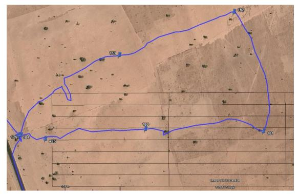
**Fig. 13.** The grid with the black lines gives the pre-selected  $plot(250 \times 25 \text{ m each})$  for site "a25". The blue line shows the actual GPS-track. The waypoints indicate where the data were split up into five different transects being each 250 m long and 50 m wide.
