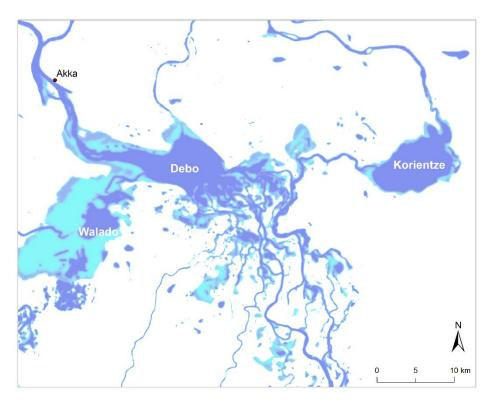
Fig. 25. The central lakes (Debo, Walado and Korientzé). The water coverage is shown for the range 0 to 140 cm at Akka; 0 = dark blue, 140 = greenblue, with intermediatecolours for the classes inbetween.
