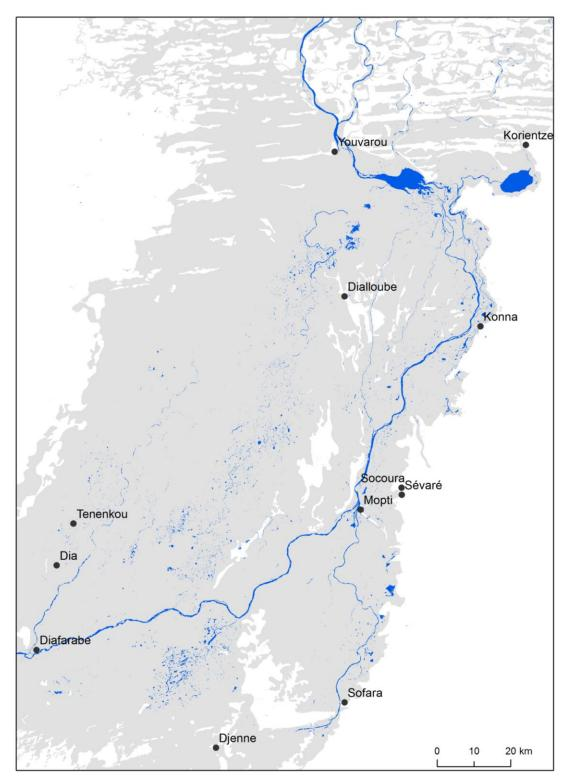
Fig. 24. The water coverage on 8-7-1985, when the water level in Mopti was 137 cm and in Akka -2 cm.
