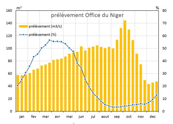
**Fig. 5.** The water taken from the Niger (m<sup>3</sup>/s) by Office du Niger near the Markala dam at point A, averaged for ten-day periods; 2000-2013. Data of Office du Niger. The yellow bars give the water intake as m<sup>3</sup>/s (left axis) and the blue line the water intake as % relative to the river flow at Koulikoro three days before (right axis). The lag of three days is based on the average difference between the timing of the peak flow in Koulikoro and Markala.
