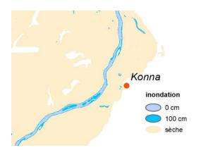
Fig. 29. What remains of the Niger River near Konna (from 20 km upstream to 10 km downstream of Konna) when the water level in Akka declines from 100 cm (light and dark blue) to 0 cm (light blue). At a water level of 0 cm, many rock and sandbanks near Konna are uncovered and the boats have to manoeuvre between the banks. Note that the map shows the water coverage independent of depth, even if the water depth is some cm. Source: Zwarts (2012).
