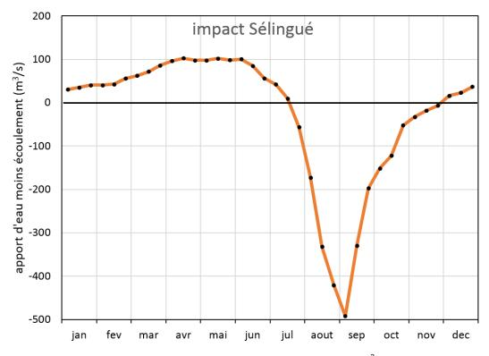
**Fig. 4.** The impact downstream of the Sélingué reservoir on the river flow (m<sup>3</sup>/s), calculated as the difference between the inflow into the reservoir and the outflow from the reservoir, averaged for ten-days periods; 1982-2013. Data of EDM. To empty the lake, water is released from early December to mid-July (outflow larger than inflow). The lake is filled from late July to late November (inflow larger than outflow).
