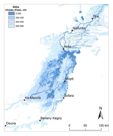
**Fig. 2.** The hydrometric stations in the Inner Niger Delta relevant for this study. The different blue colours show the area being inundated at different flood levels at Akka.
