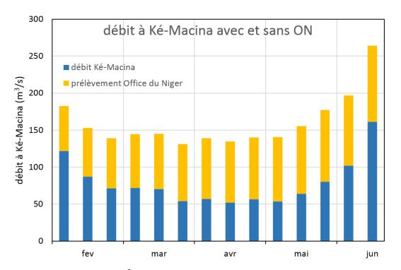
**Fig. 7.** The actual river flow (m<sup>3</sup>/s) at Ké-Macina (blue bars), between early February and mid June, averaged for ten days periods; 2000-2013. The yellow bars show the water taken from the Niger at Markala. The top of the yellow bars shows the river flow without water intake by Office du Niger.
