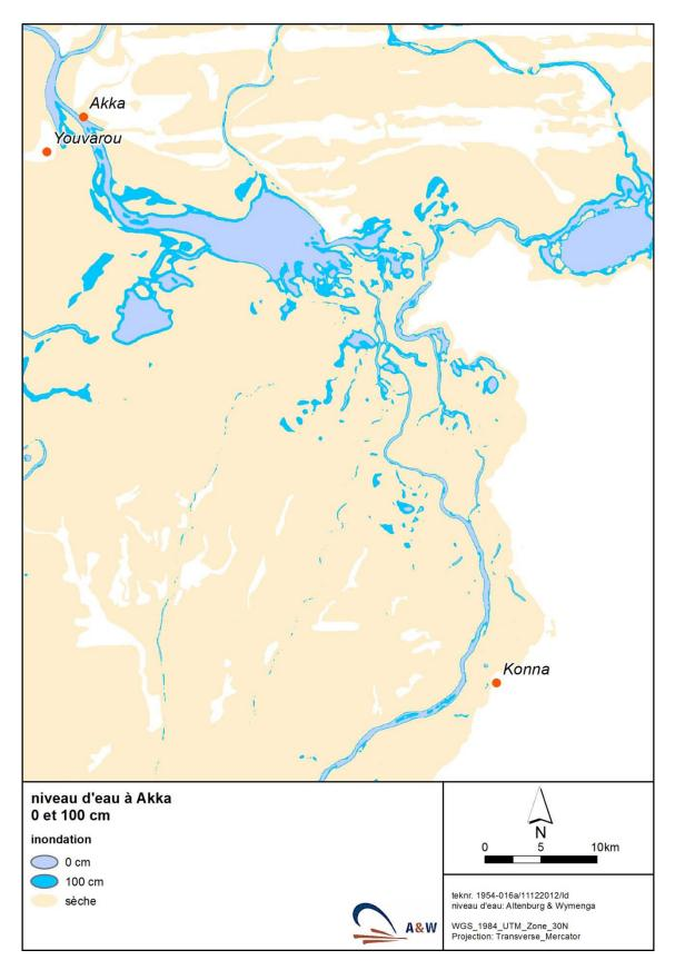
Fig. 8. The flooded area at water level of 0 or 100 cm at the gauge of Akka compared to the total inundation zone at a high flood of about 600 cm (Fig. 3; yellow). A selection has been made for the area between Akka and Konna. Note that a water level of 100 cm all floodplains are already dry, except the shallow borders of Lac Debo.
