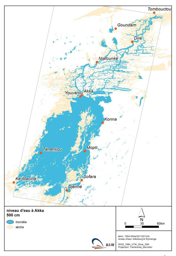
Fig. 4. The flooded area at a water level of 500 cm at the gauge of Akka (blue; total surface 17,313 km<sup>2</sup>) within the oblique rectangle, compared to the total inundation zone at a high flood of about 600 cm (Fig. 3; yellow).
