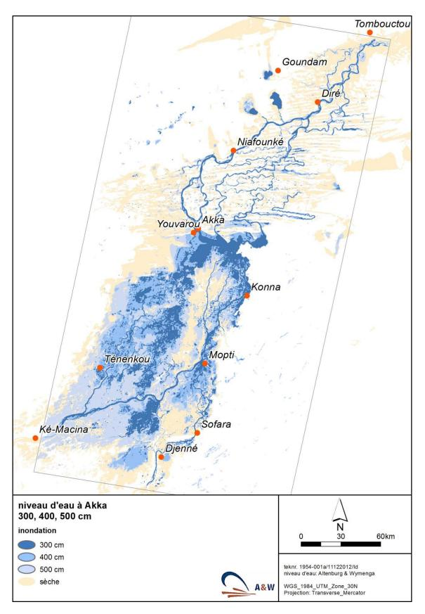
Fig. 7. The flooded area at water level of 300, 400 or 500 cm at the gauge of Akka (data from Fig. 4-6) (blue) within the oblique rectangle, compared to the total inundation zone at a high flood of about 600 cm (Fig. 3; yellow).
