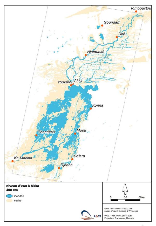
Fig. 5. The flooded area at a water level of 400 cm at the gauge of Akka (blue; total surface 9777 km<sup>2</sup>) within the oblique rectangle, compared to the total inundation zone at a high flood of about 600 cm (Fig. 3; yellow).
