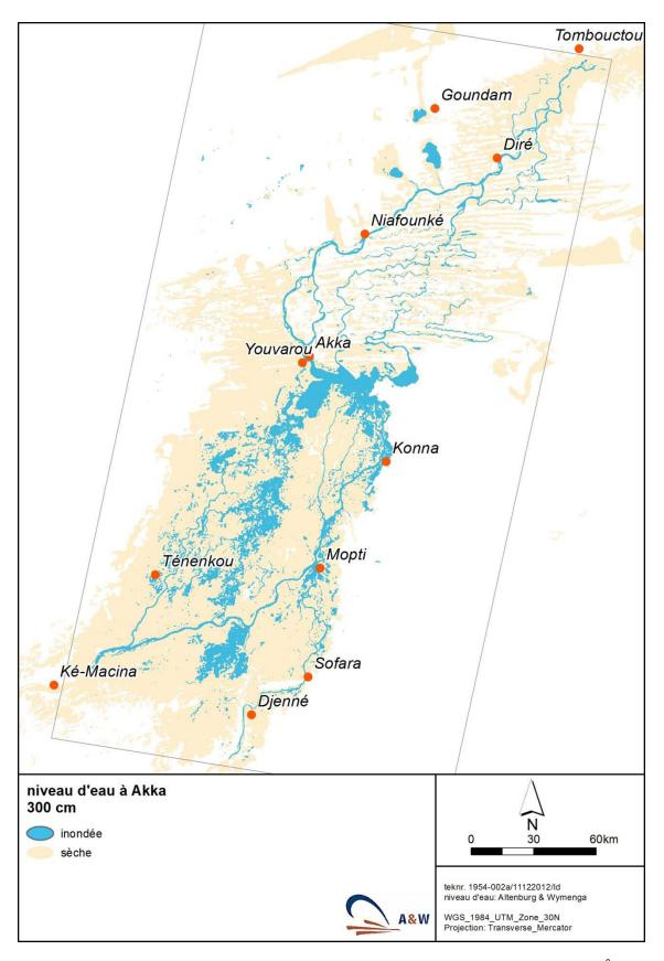
Fig. 6. The flooded area at a water level of 300 cm at the gauge of Akka (blue; total surface 4832 km<sup>2</sup>) within the oblique rectangle, compared to the total inundation zone at a high flood of about 600 cm (Fig. 3; yellow).
