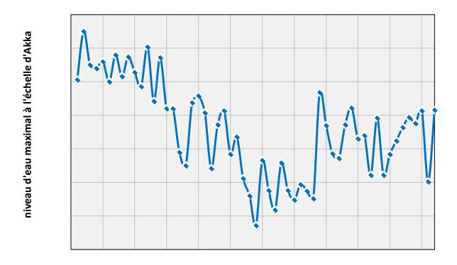
Fig. 2. The annual peak flood level in the Inner Niger Delta, measured on the gauge of Akka, has varied between 336 cm (in 1984) and 625 cm (in 1957) during the last 60 years; data from DNH.
